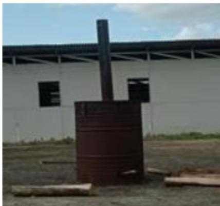
Gambar 3. Drum kiln tertutup/pirolisis
