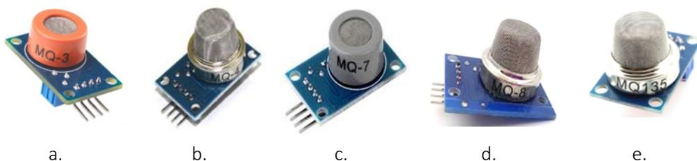
Gambar 2. Sensor emisi gas a. sensor CO<sub>2</sub>, b. sensor NO<sub>x</sub>, c. sensor CO, d. sensor HC, e. sensor asap
