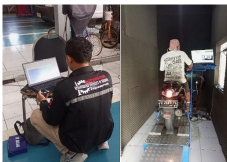
Gambar 2 Proses re-mapping ECU dan dynotest
